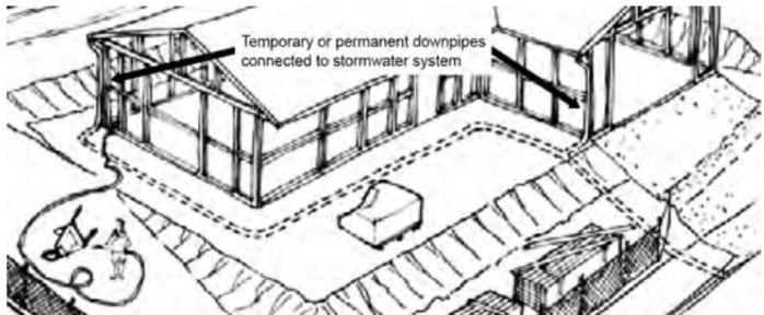
**2. Early drainage connection.** Connect downpipes and other drainage to the stormwater system as soon as the roof is on and / or other impervious surfaces are constructed, such as driveways, parking areas, or the building slab. Temporary flexible downpipes can be useful until permanent pipes and drainage system is in place.
