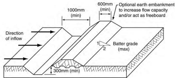
**1. Diversion drain.** The drain channel must be at least 150 mm deep with a curved shape that will be site specific. Stabilise the flow path to protect it from scour by lining the drain with matting or rock. If dispersive soils are present, create diversion drains by building soil berms instead of digging.
