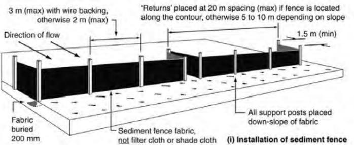
**4. Sediment fences.** Install parallel to the contour with ends angled upwards. Bury fabric 200 mm deep. Join sections of fabric at a support post with a 2 m overlap. Ensure fabric is securely attached to all support posts. Not suitable for concentrated flow paths, creeks, or major drainage lines.
