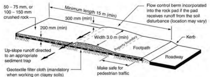
**3. Stabilised site access.** Stabilised access is from the site boundary to a formal stockpile area or work site; minimum length for small developments is 10 m. Strip at least 150 mm of topsoil, cover with geotextile then a 200 mm thick pad. Divert water from this control to appropriate sediment controls.
